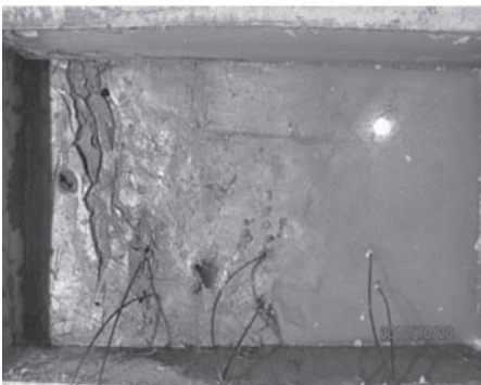
Figure 3. Soil surface of soil layer after anaerobic fermentation (the holes are formed by \text{CH}_4 drainage).
