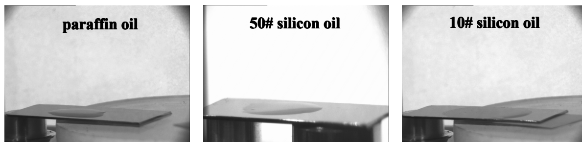
图 4: 不同液滴在迁移过程中的接触角滞后现象 Fig.4 The contact angle hysteresis phenomenon of different droplet in the migration process
