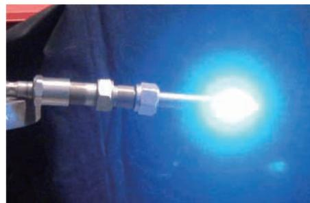
Fig. 2 Discharging of 50J/pulse spark plug
