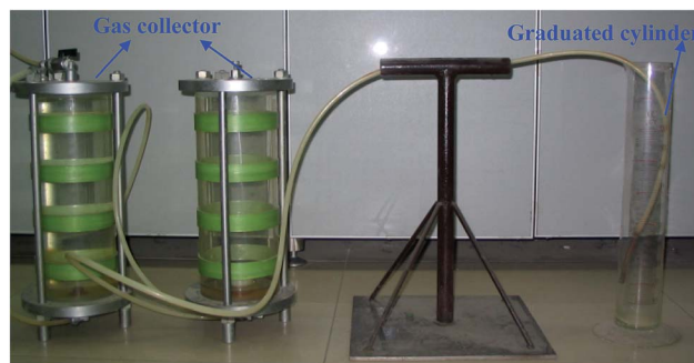
Fig. 5 Gas collection system.
