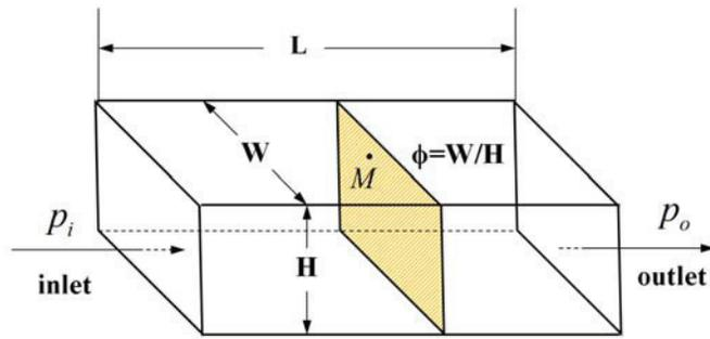
FIGURE 1. Schematic of micro-channel with rectangular cross section.
