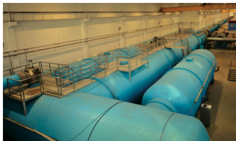
Fig. 1 Photo of long-test-duration hypervelocity detonation-driven shock tunnel viewing from its vacuum system
