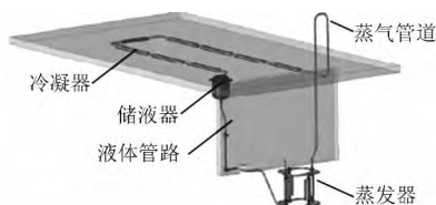
图 1 月球重力驱动的两相流体自然循环系统布局 [1] Fig. 1 Layout of a closed two-phase natural circulation system driven by lunar gravity [1]
