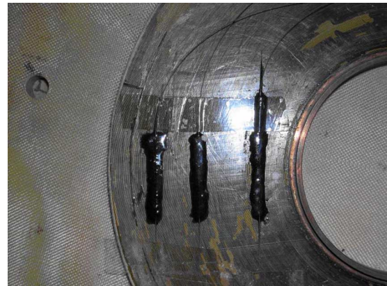
Fig. 6. Experiment setup by FBG for high temperature superconducting coil.
