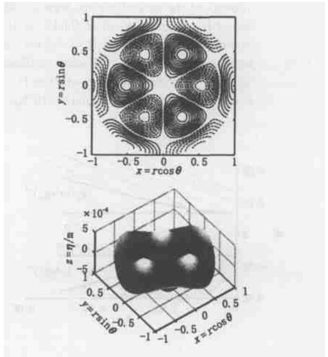
1(b) The forced frequency  $f = 10.92$  Hz, the mode of surface wave is (3, 2)
