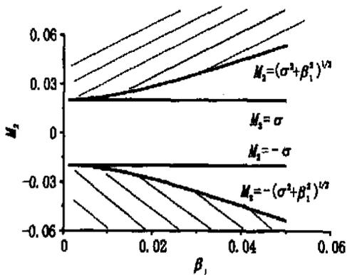
2(a) Unstable region determined by damping coefficient  $\beta_1$  and excited coefficient  $M_2$  ( $\sigma = 0.02$ )
