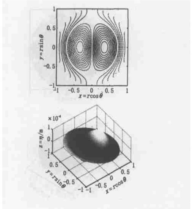
1(a) The forced frequency  $f = 8.73$  Hz, and the mode of surface wave is (1, 2)
