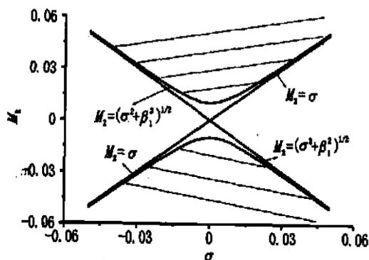
2(b) Unstable region determined by frequency difference coefficient  $\sigma$  and excited coefficient  $M_2$  ( $\beta_1 = 0.01$ )
