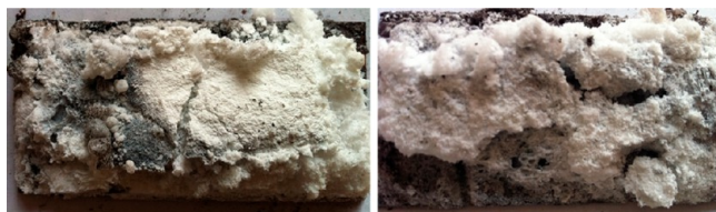
a. The surface of the char layer b. The internal part of the char layer
