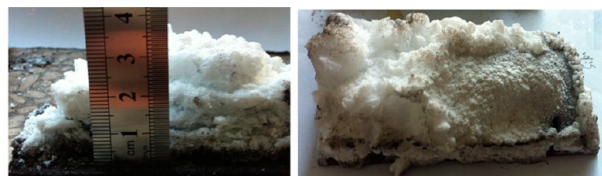
a. The char layer of the original sample b. The char layer of the 8-h corrosion sample
