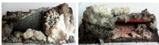
a. The surface of the char layer b. The side view of the char
