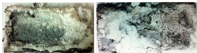
a. The surface of the char layer b. The internal part of the char layer
