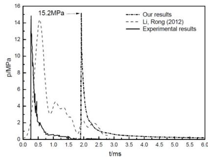
Figure 2: Pressure-time curve at 3m from the charge center. The spherical shaped charge weighted 1kg is detonated 5m under the water surface. The dot dash line is our result, while the dash line and solid line are the simulation results and experimental results, respectively, from Ref. [6]
