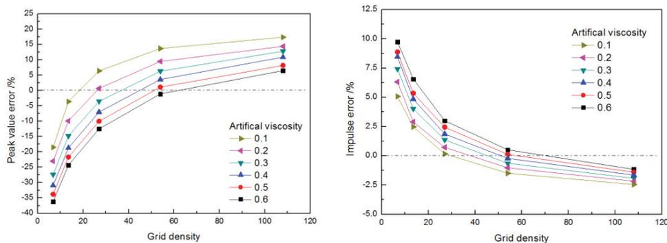
Figure 1: Influences of the grid density (element numbers in a characteristic length of the charge) and artificial viscosity. (a) and (b) are the peak value and impulse errors, respectively. The reference values marked as dot dash line are the values calculated according to Cole's similarity law for UNEX shock [4].
