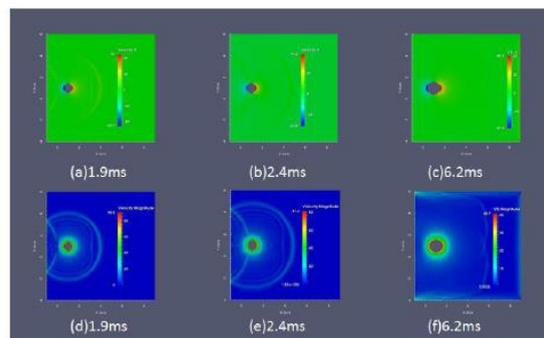
Figure 4: Interaction between the reflected shock and the expanding bubble (horizontal slices). (a)-(c) are the x component of velocity; (d)-(f) are the absolute speed. The round in the calculation region is the explosion product, i. e. the explosion bubble. The rigid wall is at the left boundary of the computational domain.
