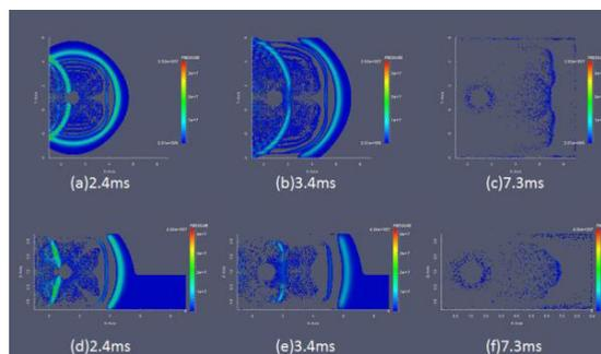
Figure 5: UNEX pressure field. (a) - (c) are horizontal slices passing through the neutral axis of the charge, while (d)-(f) the perpendicular slices. The domain where pressure lower than the hydrostatic pressure of the charge centroid is omitted.
