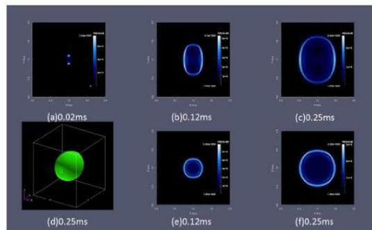
Figure 3: Underwater shock generated by a cylindrical shaped TNT. The charge is placed 2m away from a rigid wall, 10m below the water surface; it is 0.5m long with density 1580 kg/m<sup>3</sup> and weight 4kg. (a) - (c) are horizontal slices passing through the neutral axis of the charge, while (e)-(f) the perpendicular slices; (d) is the 3D profile of the shock.
