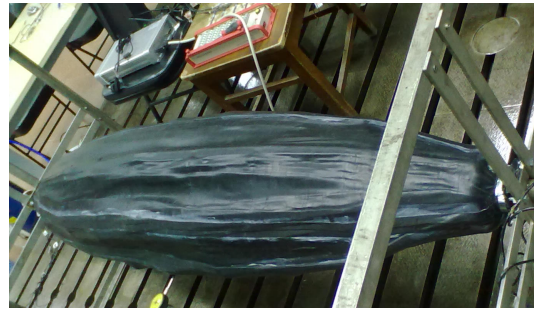
图 8 橡胶材料飞艇模型实物图 Fig.8 Airship test model with rubber material
