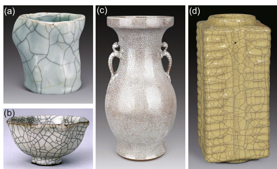
Figure 9 (Color online) Ge Kilns. (a) Brush pot; (b) octagonal bowl; (c) double-ear porcelain vase; (d) yellow glazed square vase. (a) and (b) show large cracks appearing on the smaller ceramics, (c) shows typical uniform small cracks appearing on larger ceramics, and (d) shows ice crack.
