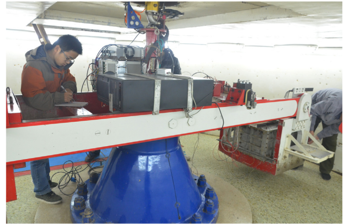
Fig. 1. The centrifuge and the model box.
