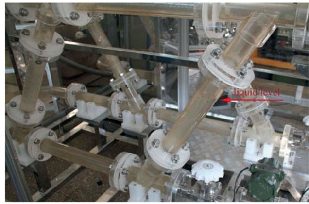
Figure 5. The liquid level in the Y-junction tubes.
