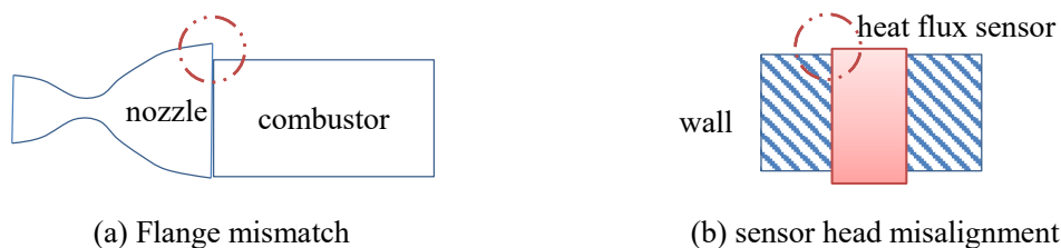
Figure 8 Schematics of installation and machining error
