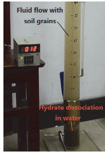
(b) fluid flow with soil grains during dissociation
