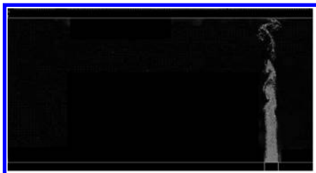
A: subsonic free jet of one hole
