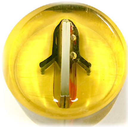
Fig. 6. The surface of a weld cross-section after grinding and polishing processes.
