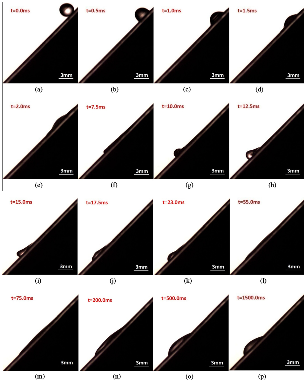
Fig. 3. Sequence of images of the water droplet impact process at an inclined angle of 45.0^\circ ( T_w = -10.0^\circ\text{C} ).
