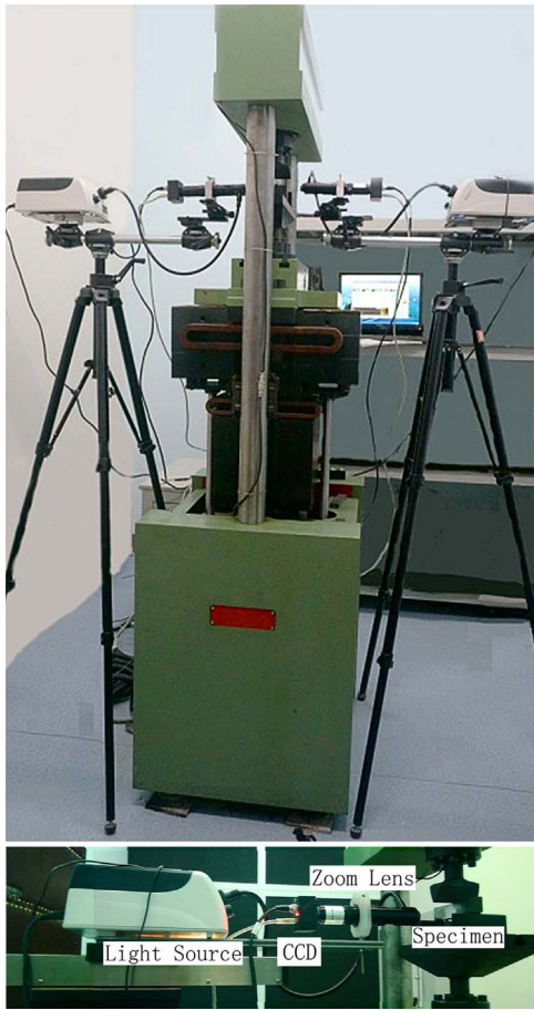
Fig. 2. Electromagnetic fatigue testing machine and in-situ optical observation system.
