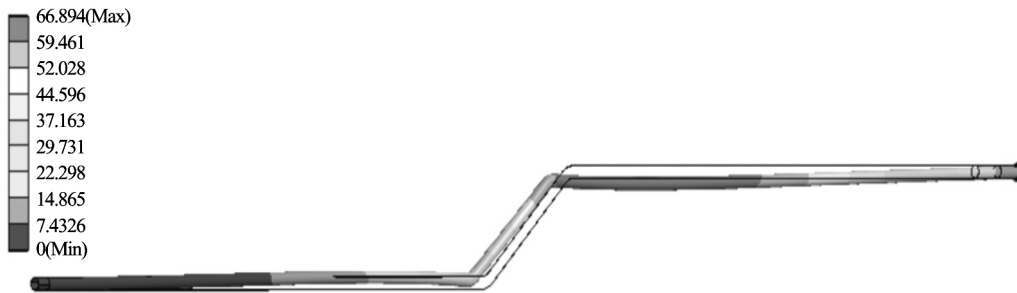
图6 Z形补偿管道变形图 Fig.6 Deformation figure for pipe with Z compensation
