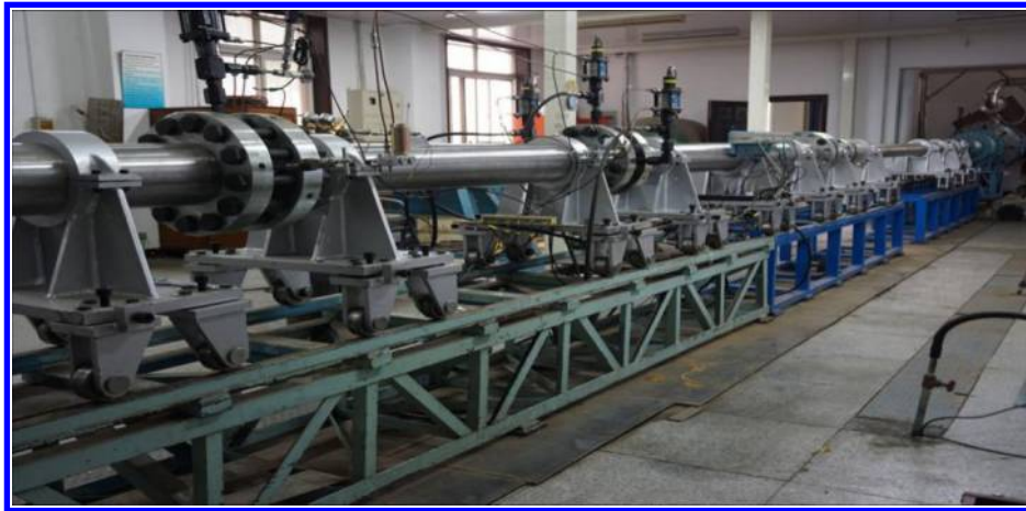
Figure 1. Photo of JF-X detonation shock tunnel
