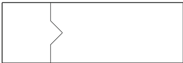
Fig. 5 Computational domain and initial condition in 2D detonation wave
