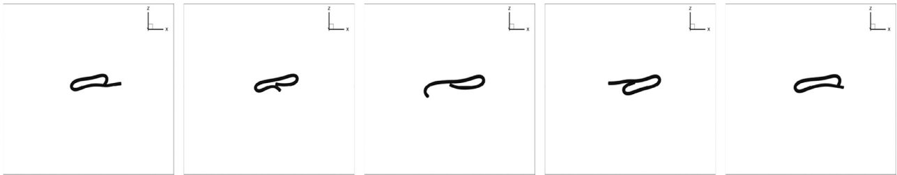
Fig. 4. A coiled rotation without entanglement at \kappa = 8321.57 . The fiber size is (1, 1, 100) and simulation box size is (255, 63, 127).
