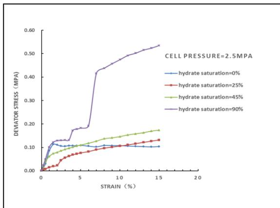
Fig.6 Stress-strain curves of clay sediment samples containing different hydrate saturation after hydrate dissociation under  $\sigma_3 = 2.5\text{MPa}$  conditions
