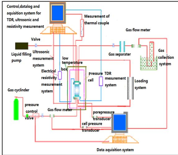
Fig. 1 Sketch of the tri-axial compression test equipment for hydrate-bearing sediment
