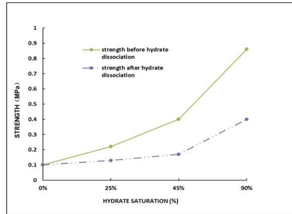
Fig.7 Undrained shear strength of clay containing hydrate before and after hydrate dissociation under  $\sigma_3 = 2.5\text{MPa}$  conditions
