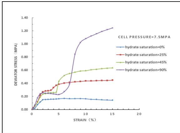
Fig.5 Stress-strain curves of clay sediment samples containing different hydrate saturation under  $\sigma_3 = 7.5\text{MPa}$  conditions
