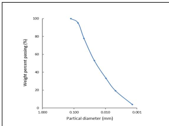
Fig.2 Grain size distribution of clay sediment
