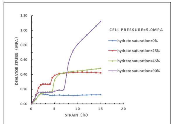
Fig.4 Stress-strain curves of clay sediment samples containing different hydrate saturation under  $\sigma_3 = 5.0\text{MPa}$  conditions
