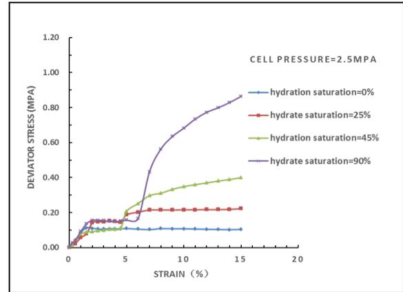
Fig.3 Stress-strain curves of clay sediment samples containing different hydrate saturation under  $\sigma_3 = 2.5\text{MPa}$  conditions
