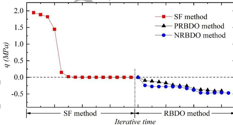
Fig. 12. Limit state function ( $q$ ) with respect to the iterative time for the two methods
