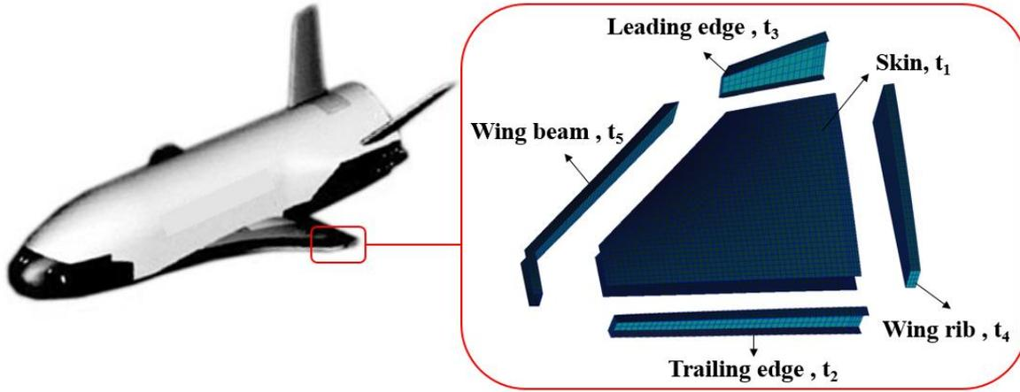
Fig. 16. Overall optimization model of wing structure.
