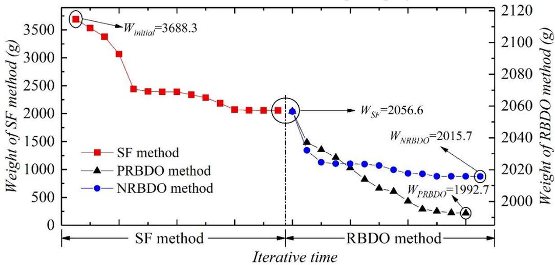
Fig. 9. Convergence curves of the two methods for the two-bar truss.
