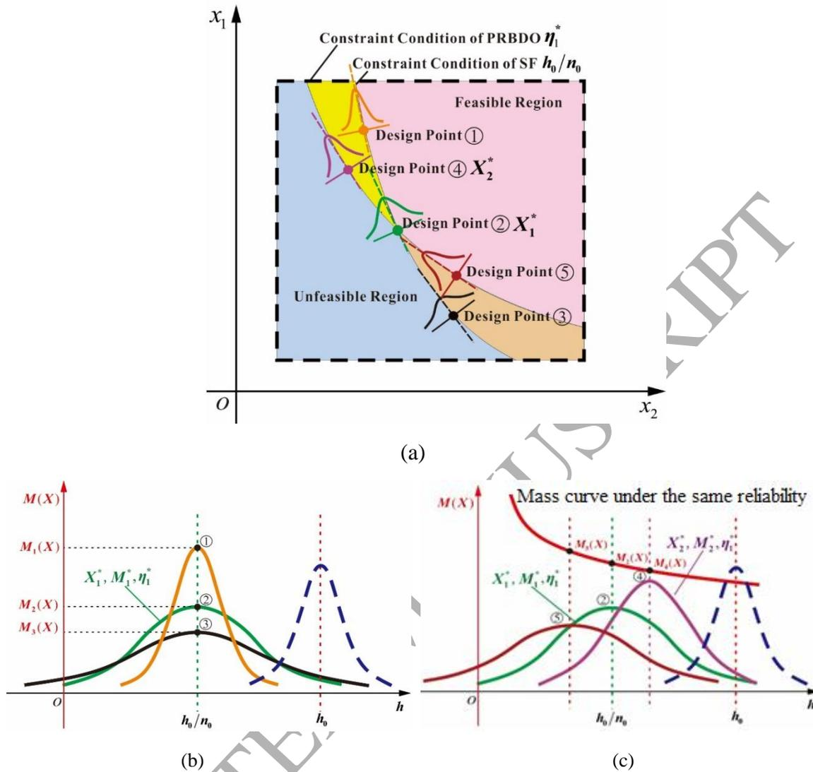
Fig. 4. Comparison of the optimization process between the PRBDO and SF methods: (a) Feasible region of the two methods, (b) Searching process of the optimal design point of the SF method, (c) Searching process of the optimal design point of the PRBDO method.
