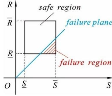
Fig. 1. Nonprobabilistic set-theoretic stress–strength interference model.
