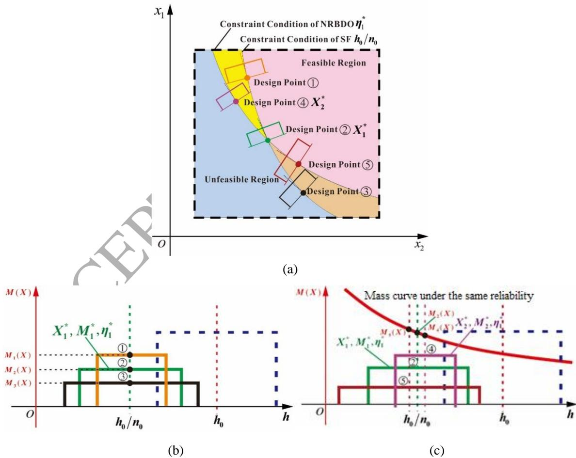
Fig. 5. Comparison of the optimization process between the NRBDO and SF methods: (a) Feasible regions of the two methods, (b) Searching process of the optimal design point of the SF method, (c) Searching process of the optimal design point of the NRBDO method.
