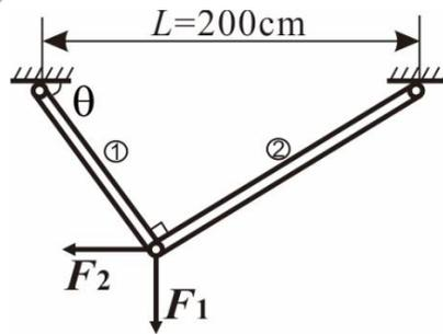
Fig. 8. A two-bar truss structural system.
