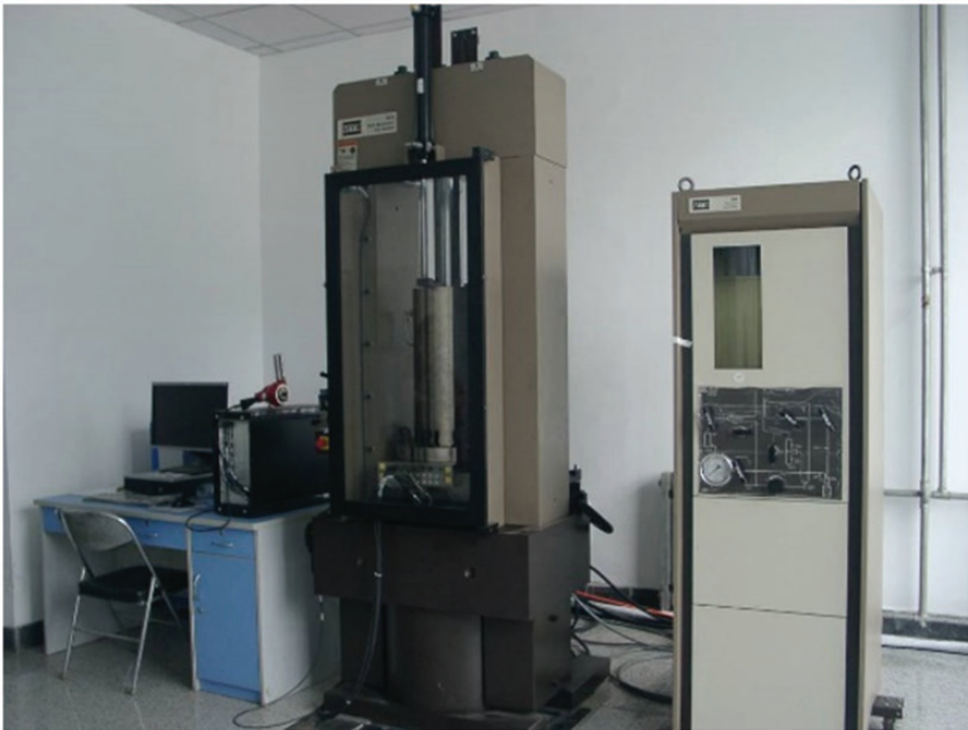
Figure 1. MTS815 experimental device system.
