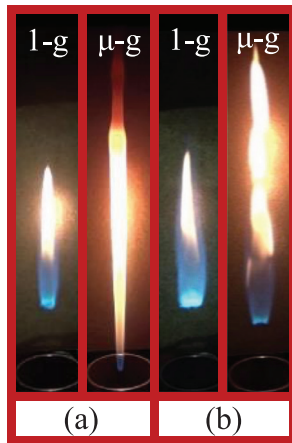
Fig. 4. Flames images in normal- and micro-gravities for (a) ( U_F [m/s], U_A [m/s]) = (6.37, 0.5) and (b) (10.6, 0.5).
