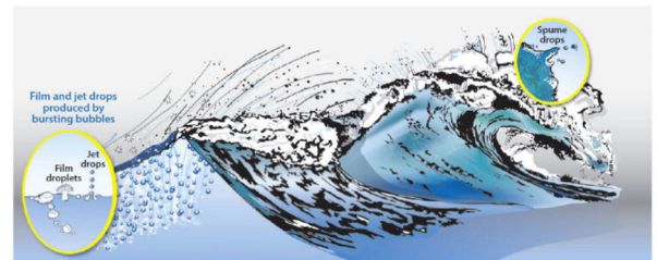
图1 波浪破碎生成的气泡与海面的相互作用 [33] Fig. 1 Interaction between bubbles and free surface owing to breaking wave [33]
