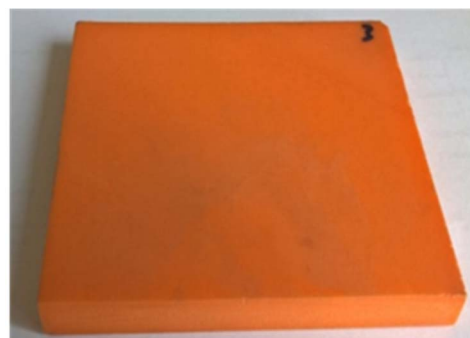
图 2 纳米微球增强聚氨酯泡沫材料样品 Fig.2 Samples of nano-microsphere enhanced polyurethane foams
