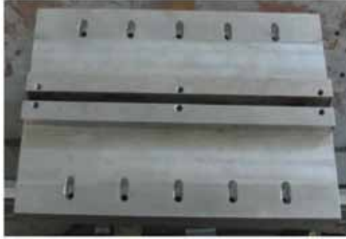
FIGURE 2 Photograph of the fixture used for the fibre laser butt joint welding tests.
