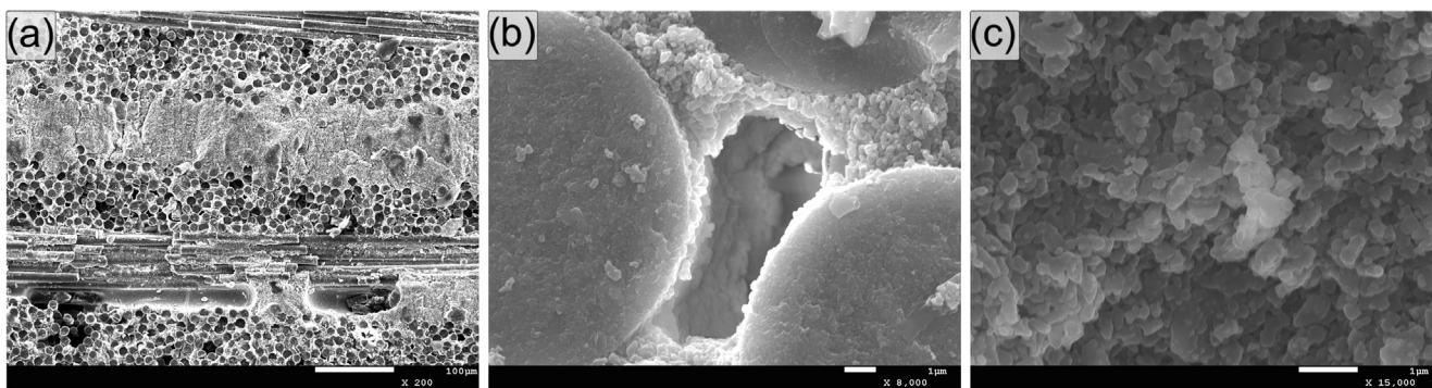
Fig. 2. The original 2-D woven ox/ox-CMCs: (a) overview, (b) fiber and matrix, (c) the porous matrix is evident.
