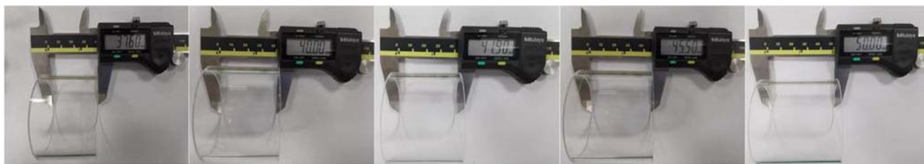
Fig. 4 The discharge chamber with different length quartz tubes
