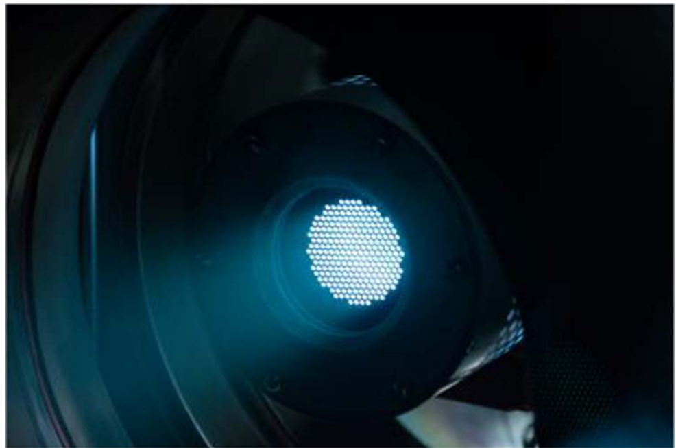
Fig. 6 The discharge in RIT-5
