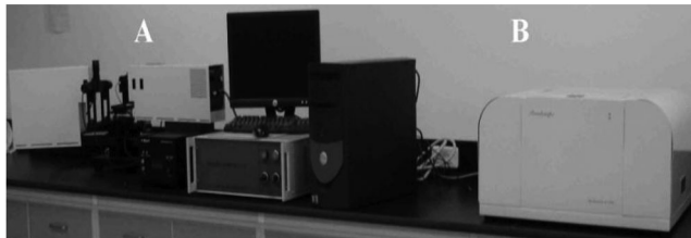
Figure 1. The illustration of Bie system. (A) imaging ellipsometry system and (B) array fabrication and microfluidic system.
