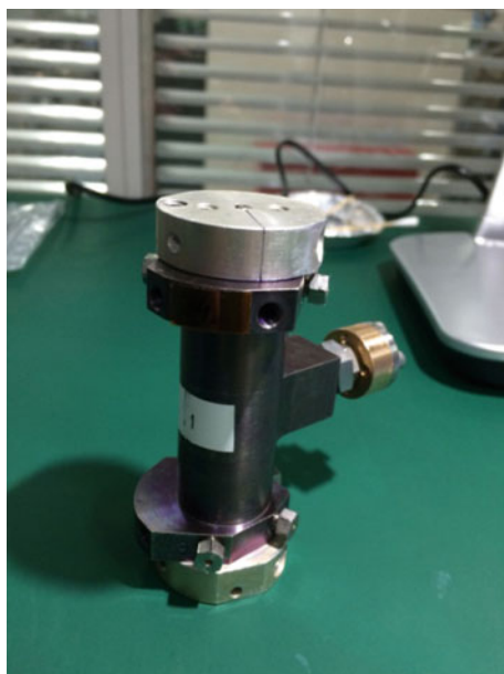
Fig. 1 One of the HP cells flown in SJ10 before integration in its triad and in the C-Box. Note the two aluminium blocks attached at the titanium end parts
