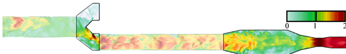
Fig. 7. Plan of the simulated instantaneous water surface in the Side A flume for the case, including the splitter. The flow discharge is equal to 1.0 \text{ m}^3/\text{s} . The color map shows the velocity magnitude in m/s, and flow is from left to right.
