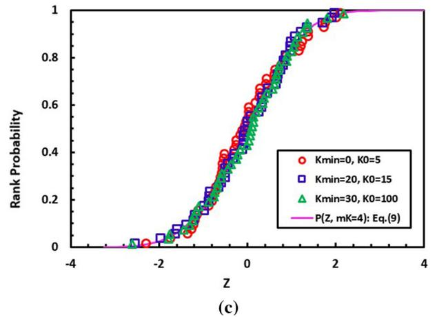
Fig. 2—Three cleavage fracture toughness distributions all with  $m_K = 4$  but different  $K_0$  and  $K_{\min}$ : (a) Raw toughness data, (b) the standardized formats with population mean and standard deviation, (c) the standardized formats with sample average and standard deviation, (d)  $\hat{m}_K$  vs number of data sets, (e) maximum likelihood estimation with all three data sets as input.
