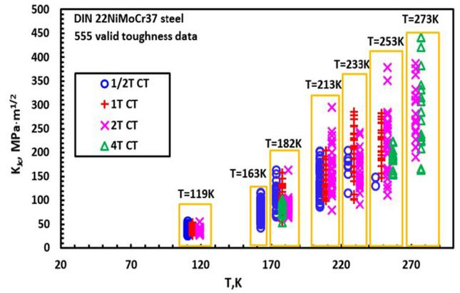
Fig. 7—All 555 valid data points of cleavage fracture toughness (Data listed in Ref. 16).
