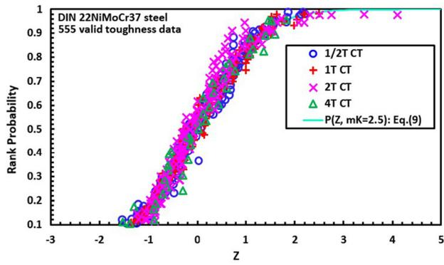
Fig. 13—Standardized distribution of cleavage fracture toughness of all CT specimens.
