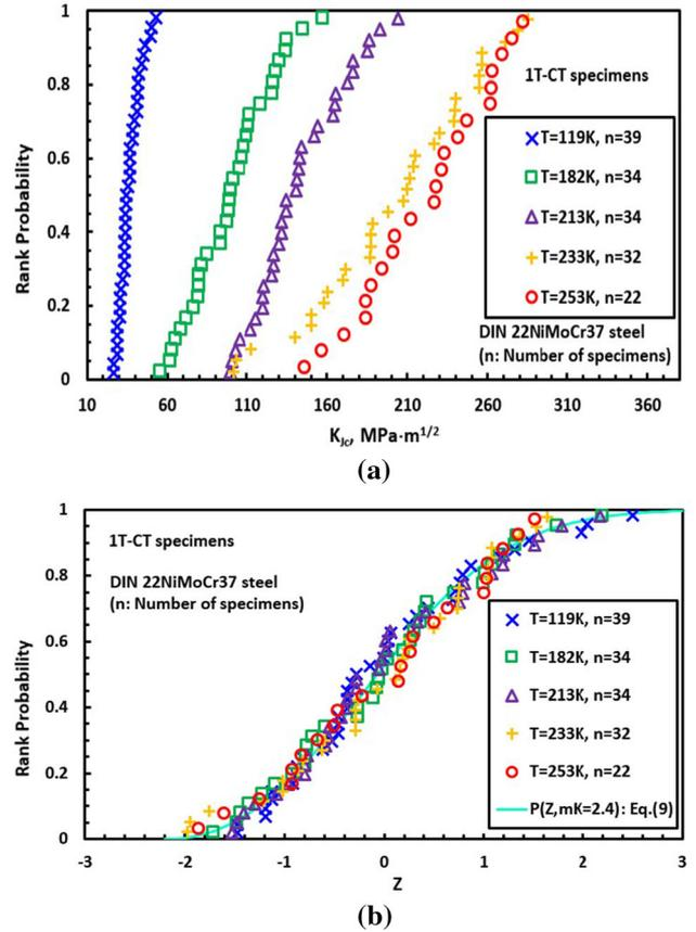
Fig. 10—Cleavage fracture toughness of 1 T CT specimens: (a) experimental data (Data listed in Ref. [16]), (b) standardized distribution of cleavage fracture toughness.
