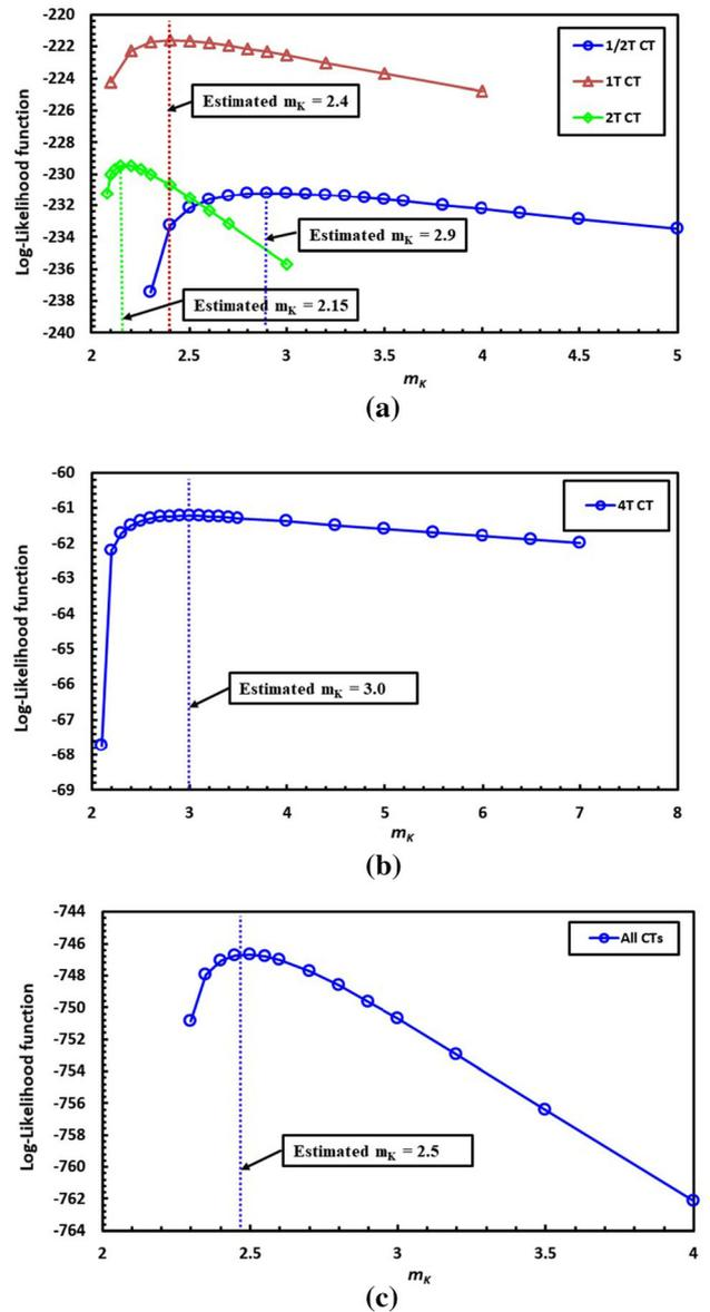
Fig. 8—Results of maximum likelyhood estimation: (a) 1/2 T CT, 1 T CT and 2 T CT specimens; (b) 4T CT specimens; (c) all CT specimens.
