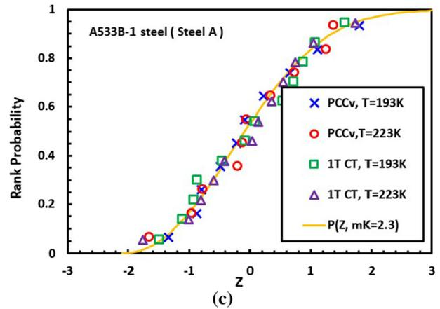
Fig. 4—(a) Experimental data of cleavage fracture toughness  $K_{JC}$  of A533B Cl.1 steel measured with 0.5 T, 1 T and 2 T specimens at 123 K (data listed in Ref. 14), (b) maximum likelihood estimate of Weibull modulus  $m_K$  using all 38 experimental data, (c) comparison of experimental  $K_{JC}$  distribution with estimation.
