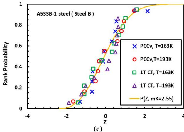
Fig. 6—(a) Experimental data of cleavage fracture toughness  $K_{IC}$  of A533B-1 steel (Steel B) at different temperatures (data listed in Ref. 15), (b) maximum likelihood estimate of Weibull modulus  $m_K$  using all 44 experimental data, (c) comparison of experimental  $K_{IC}$  distribution with estimation.
