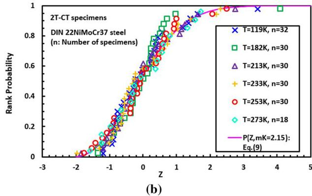
Fig. 11—Cleavage fracture toughness of 2 T CT specimens: (a) experimental data (Data listed in Ref. [16]), (b) standardized distribution of cleavage fracture toughness.
