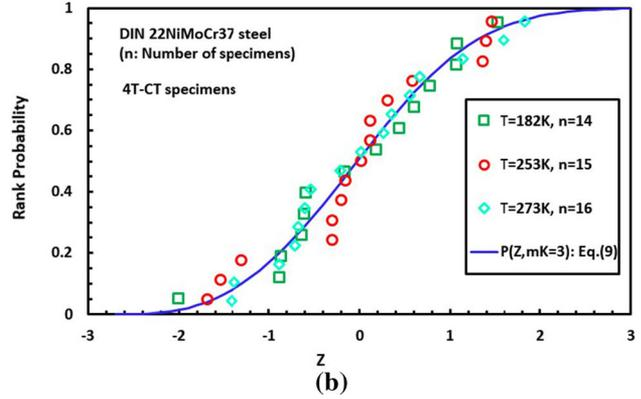
Fig. 12—Cleavage fracture toughness of 4 T CT specimens: (a) experimental data (Data listed in Ref. [16]), (b) standardized distribution of cleavage fracture toughness.
