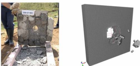
(c) 钢筋混凝土板爆炸试验和模拟 (c) Explosion test and simulation of reinforced cement panel
