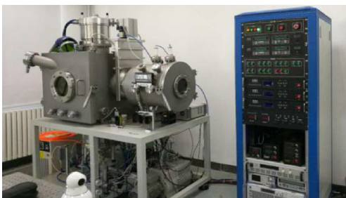
Fig. 1 Space vacuum environment ground simulation experiment platform
