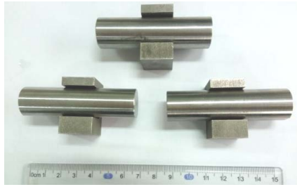
图 2 底座和拉杆模拟件的配合图 Fig.2 Assembly drawing of pedestal and tie bar
