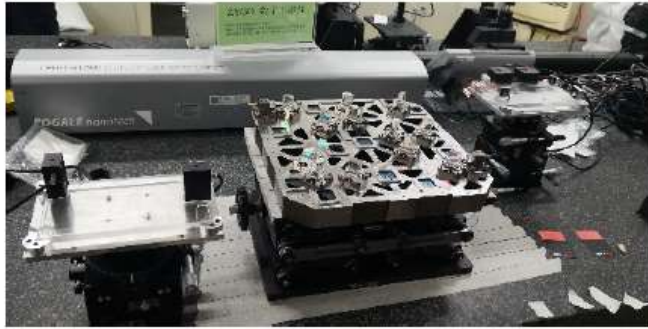
Fig. 13. Alignment of equal arm interferometer and laser frequency interferometer.
