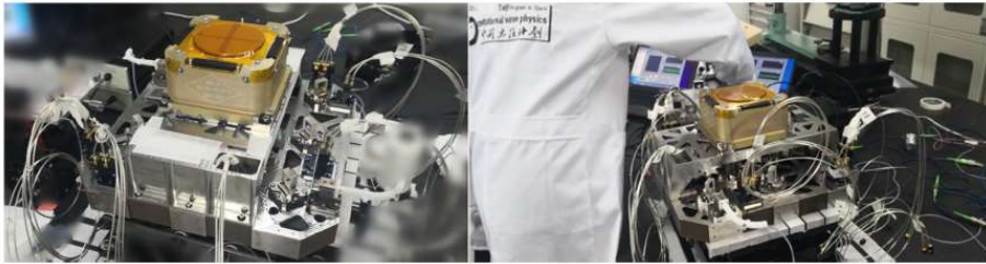
Fig. 14. Alignment of test mass interferometer.
