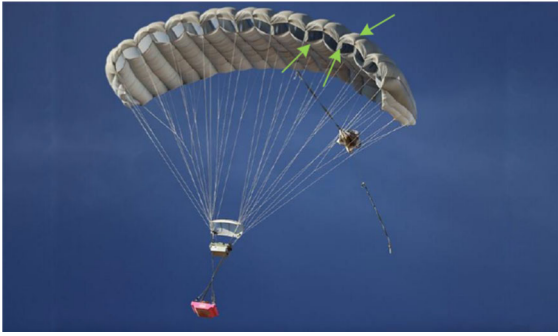
Fig. 1 Ram-air parachute side view during flight (Adapted from Airborne Systems, from https://airborne-sys.com/product/cargo-delivery-system-army-microfly-ii/ )
