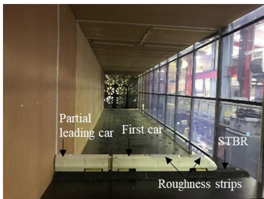
Fig. 2 Experimental set-up of the train model at a yaw angle of 90^\circ inside the wind tunnel
