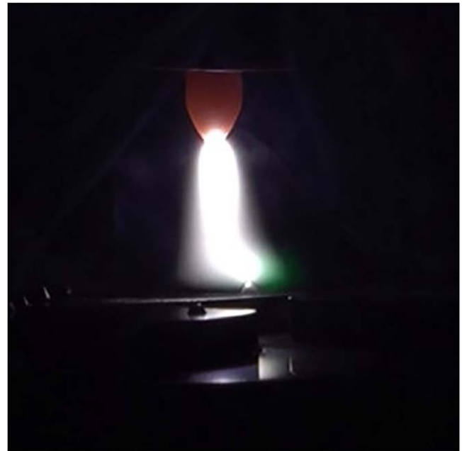
Figure 10. Experimental photo of a free burning argon arc with protrusion on anode.
