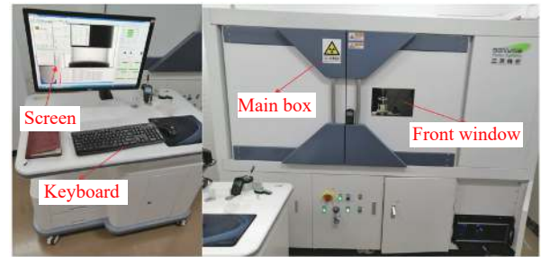
Fig. 5. High-resolution X-ray three-dimensional scanning imaging system.
