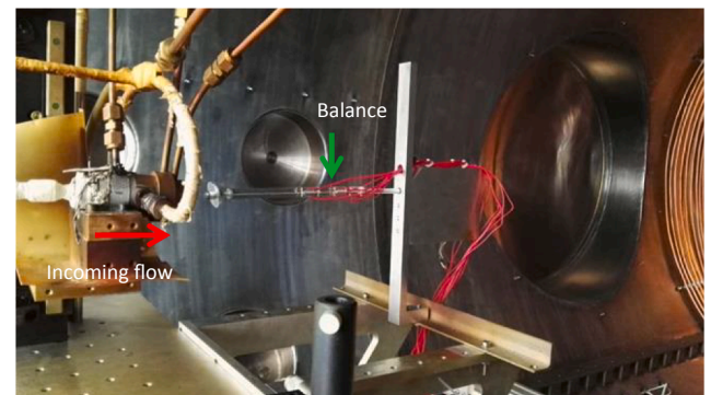
Fig. 11. In-situ experiment in the hypersonic rarefied wind tunnel.
