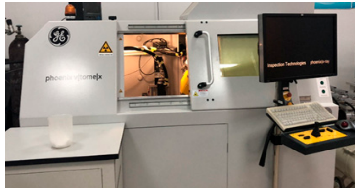
Figure 1. The integrated equipment (CT combined with triaxial apparatus). This is the overall image of the equipment. In the central window is the triaxial apparatus. The controlling and data collection system are located at right side.
