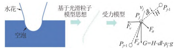
图3 (网上彩图) 基于光滑粒子模型思想的水花动力学模型分析示意图 Fig.3 (Color online) Analysis diagram of splash dynamics model based on Smooth Particle Hydrodynamics model
