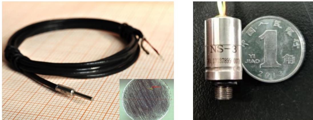
Figure 5. Type-E coaxial thermocouple heat flux sensor (left) and NS-3 pressure sensor (right).
